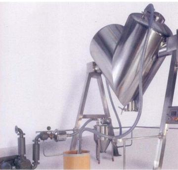
The system comprises a twin lobe vacuum duty air cooled pump, a cyclone separator, a bypass valve damper, two stage food grade silicon coated polyester filters, associated pipe lines and the food grade hose pipe with pickup device.
